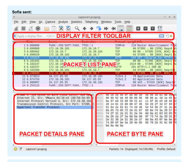
While I've highlighted and named all the main parts of the user interface, we will only be using the **Display Filter Toolbar** and **Packet List Pane** today.
